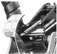
Depth Indicator for precise depth control
